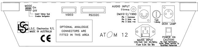
Rear panel layout of an Atom 12/24. An Atom 24/48 has provision for a second analogue output module.
