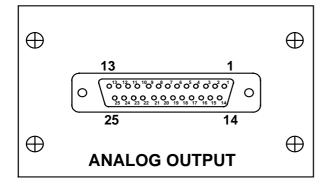
If a second DB25 connector module is fitted (to the right of the first module when viewed from the rear) it provides outputs for channels 25 to 48.
