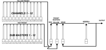
Simplified block diagram of a 12/24 Atom in **SCENE** mode.
