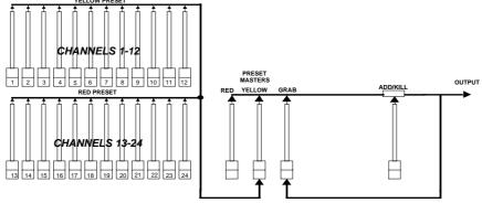
Simplified block diagram of a 12/24 Atom in Wide preset mode.
