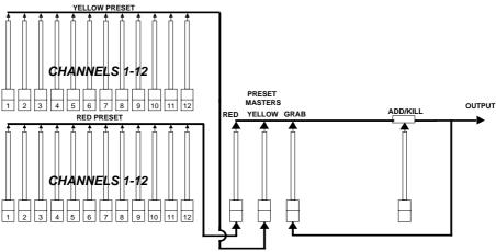
Simplified block diagram of a 12/24 Atom in **PRESET** mode.
